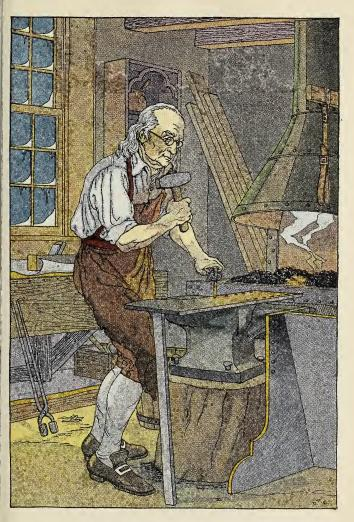
to heat iron. Red-hot iron is soft. It can be bent easily, and holes can be punched in it.
