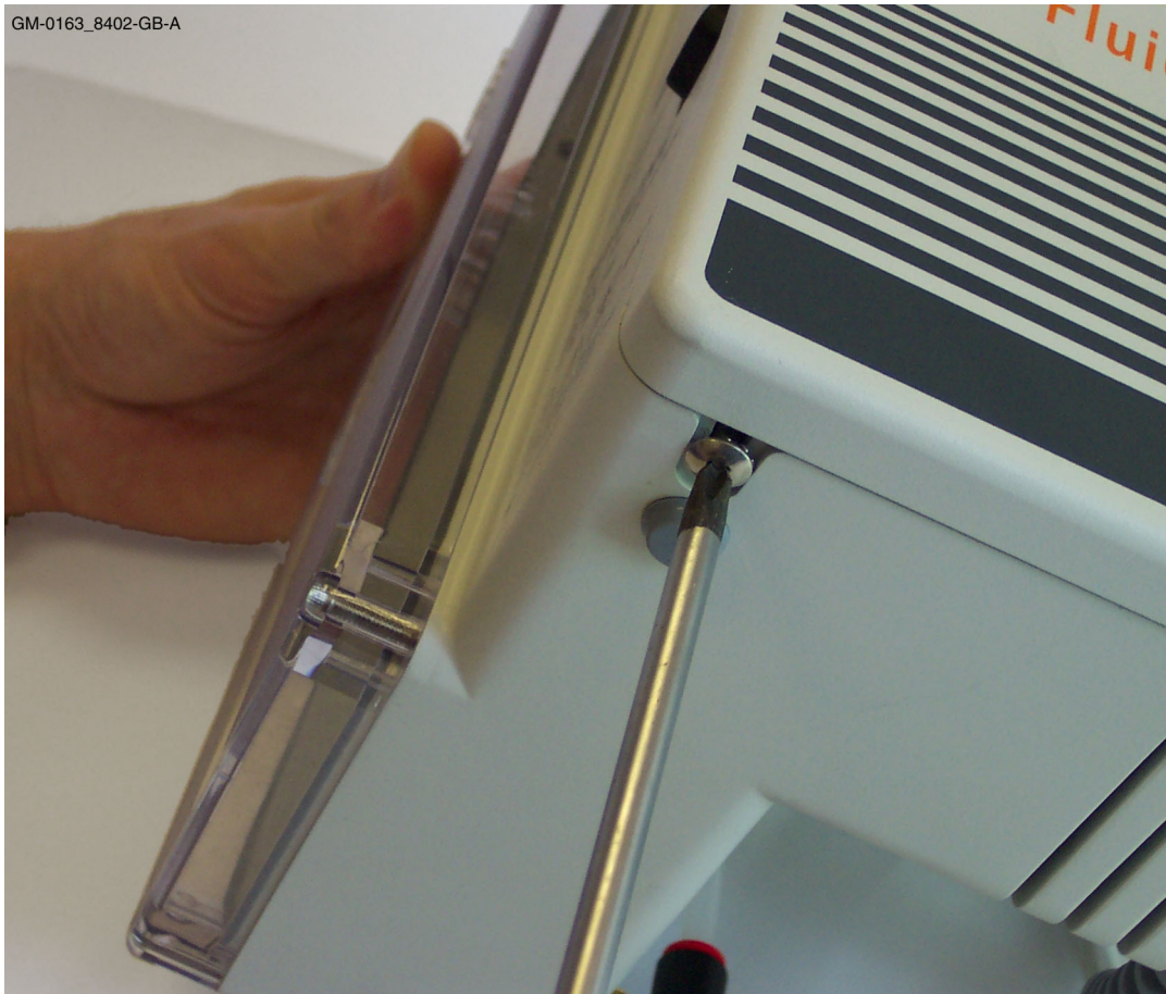
Figure 4 - 2: Loosen, but don't completely remove these screws
