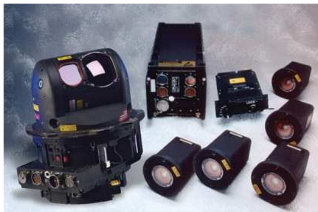
AN/AAQ-24(V) Missile Approach Warning - Missile seeker Laser blinding components
