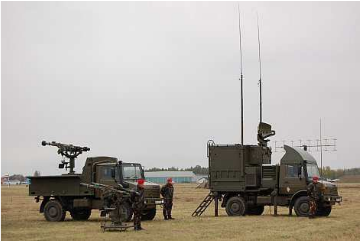
Hungarian ATLAS on Unimog, ATLAS dismantled, and MCP (Mistral Co-ordination Post)
