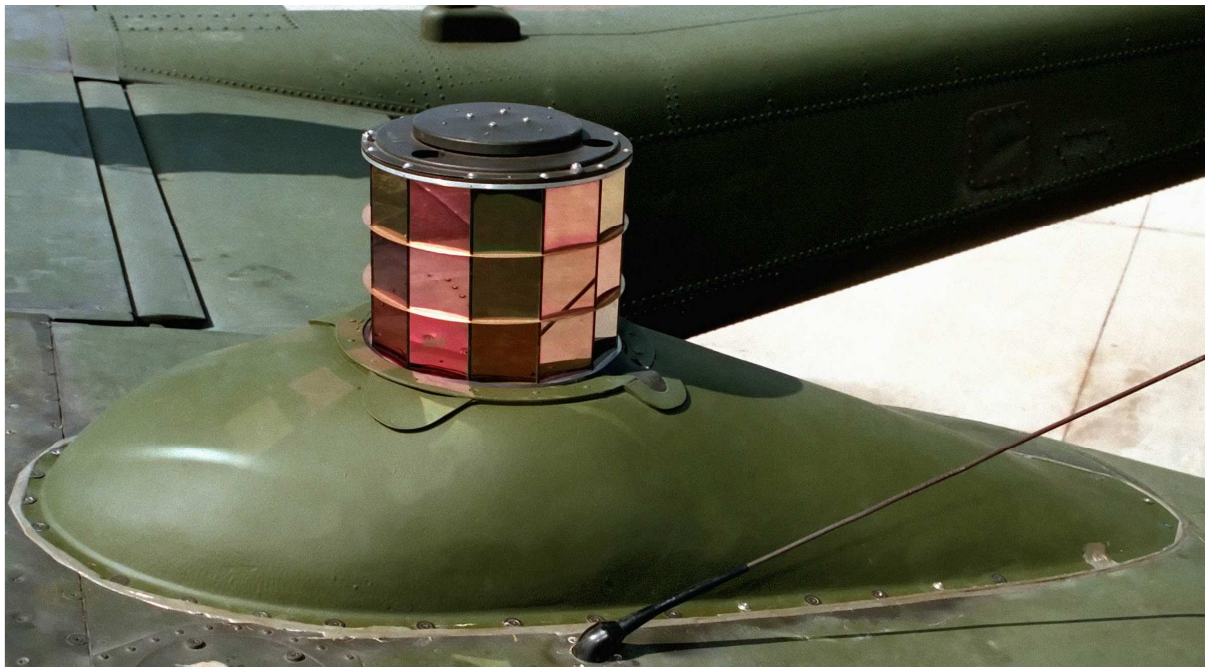
Mechanically modulated element heated to incandescence - ALQ-144
