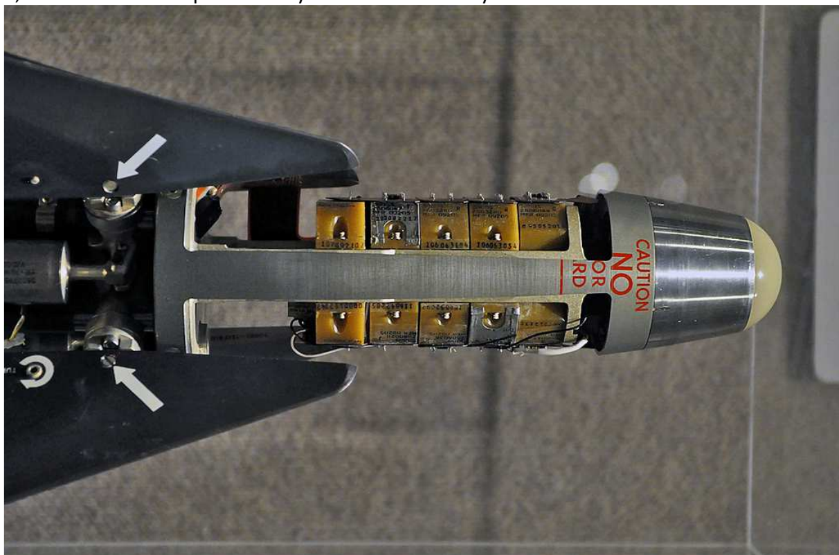
AIM-9H Sidewinder all-transistor seeker head using cordwood packaging 50
