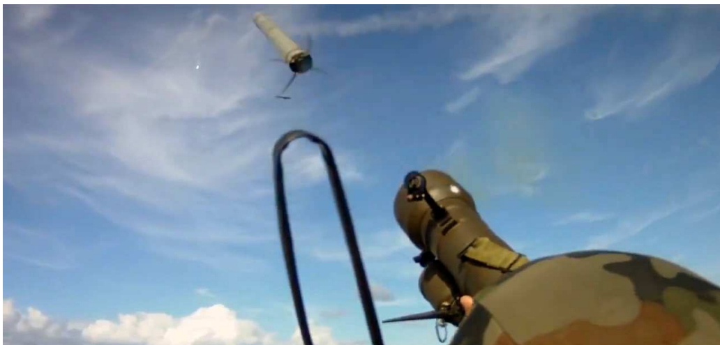
9K32 Strela-2 (SA-7 Grail) missile ejected from the launch tube towards a flare target
